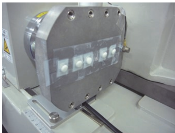
Fig. 25. Photo image of immobilized tablets on the test stage of PST-300. Blister-packed tablets were attached horizontally on the center line of test stage.
